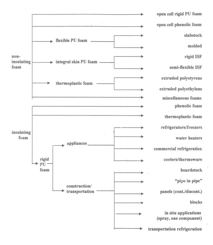
The most prevalent use of **open cell rigid PUR foam** is for packaging applications ("pour in place" foam), mostly when small lots are involved, such as in the return of repaired items. Another application is "back-foaming" of crash panels, such as automotive dashboards.
